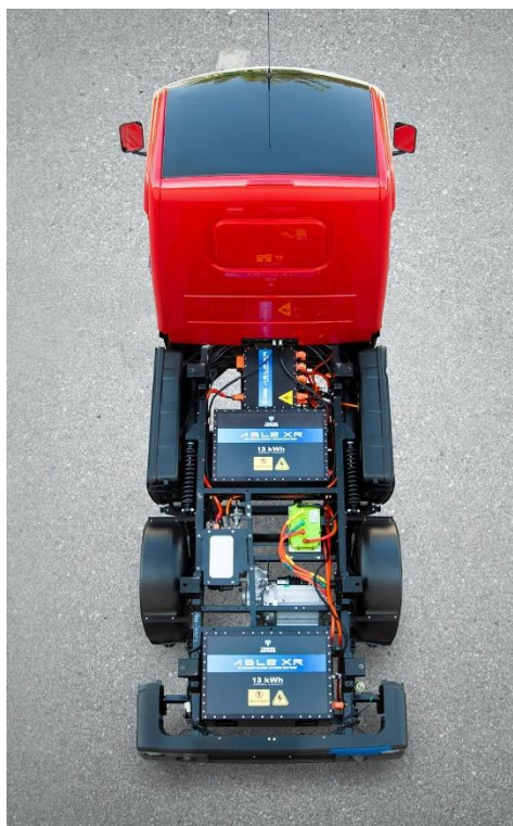
Figure 21: Placement of battery packs and electric motor of Tropos Motors utility vehicle 71
