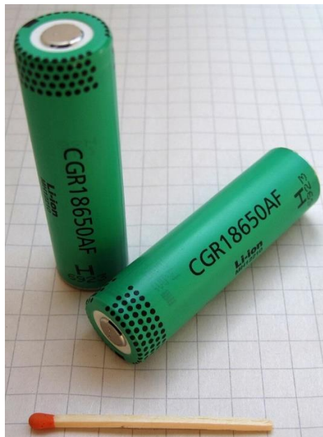
Figure 42: Example of battery cells used in a scooter battery pack 131
